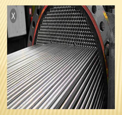
We manufacture a heat exchanger which is used to transfer heat between two or more fluids
