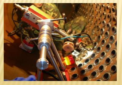
Tube expanders are devices that are used to increase the diameter of a piece of metal tubing . there are several benefits of using a tube expander with a small copper tube .
