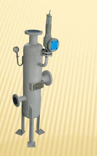
Flash Vessel is equipment used in any steam plant for flash evaporation recovery system. Usually high pressure condensate is reduced to lower pressure and is separated in the flash recovery system to prevent pollution of boiler feed tank or heat transfer surfaces
