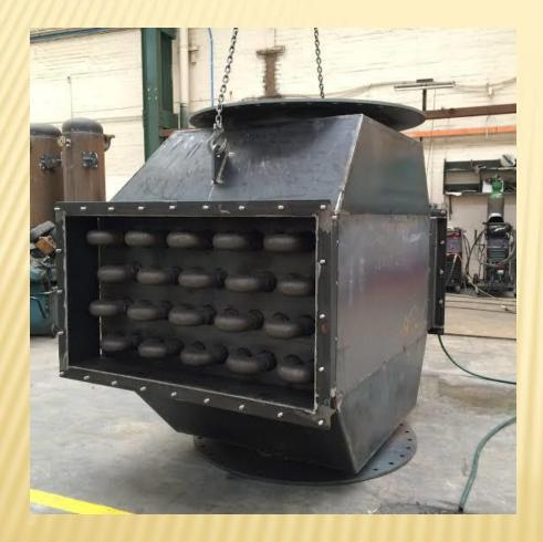
We manufacture the economizer. It is a mechanical device intended to reduce energy consumption or to perform useful function such as per heating a fluid
