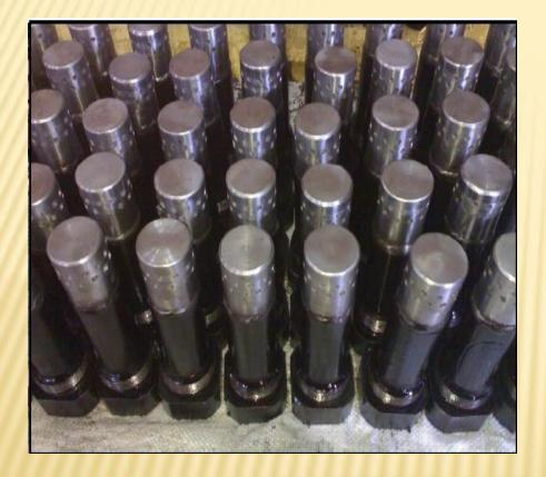
We offer a premium quality collection of Air Nozzles providing effective fluidization for optimum combustion of fuel in boiler furnace.
