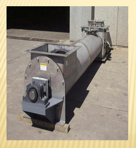
Screw feeders are available in different sizes with heat treated plate being used for making screw. This enhances the life of screw thus providing smooth and maintenance free operation of fuel feeding.
