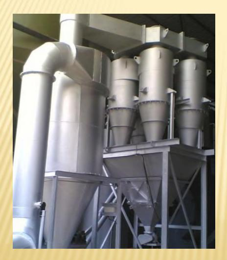
We manufacture high efficiency dust collection equipment, which not only reduces particulate emission in flue gases but also prevent smoke nuisance & helps in reducing ID fan erosion.
