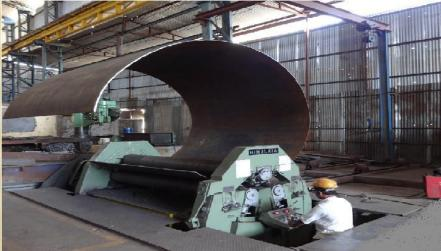
In metalworking, rolling is a metal forming process in which metal stock is passed through one or more pairs of rolls to reduce the thickness and to make the thickness uniform. The concept is similar to the rolling o dough. Rolling is classified according to the temperature of the metal rolled.
