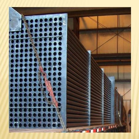
Air per-heater assemblies are designed for effective heat transfer from flue gases to fresh air. The size and dimensions of the air heater assemblies are calculated and designed in line with boiler rating.
