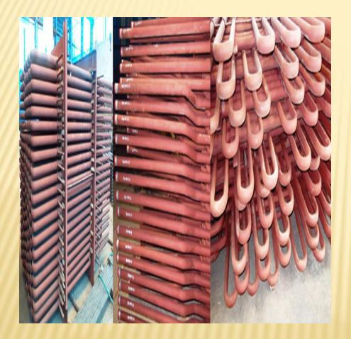
We manufacture a super heater . This is a device used to convert saturated steam or wet steam into superheated
